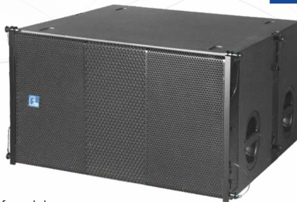
The **MLA215B** is a dual 15" low frequency enclosure designed for sub-bass reinforcement to MLA210, made of high quality plywood with polyurea waterproof paint. All rigging parts are made of aluminium alloy. The **MLA215BA** is equipped with BA2.88 digital amplifier module based on **MLA215B** to be an active subwoofer.
