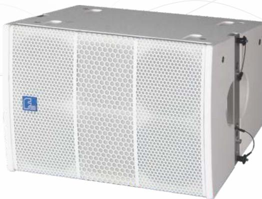
The **MLA406** is a mini line array loudspeaker for small and medium scale sound reinforcement. MLA406 is a 2.5-way design housing fitted with four 6" neodymium LF drivers and two 1" neodymium HF drivers coupled to a patent line array horn, made of high quality plywood with special environmental protection paint. MLA406A is equipped FA1.6 digital amplifier module to be active loudspeaker based on MLA406.
