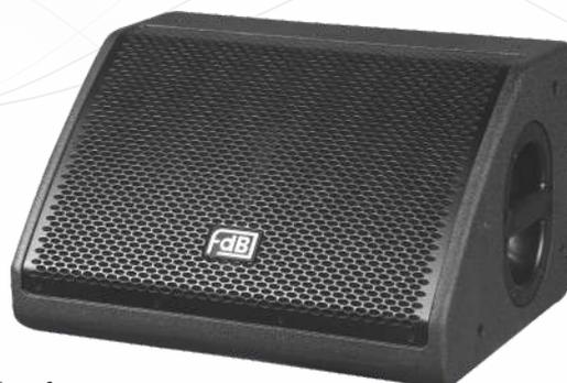
The **MR208** is a high precision and high power stage monitor, made of high quality plywood with polyurea paint. It offers a "studio monitoring" type of response, exceptional dynamic capability and very low distortion. Fitted with two 8" woofer and one 1" exit neodymium compression driver. MR208A is equipped with FA1.6 digital amplifier module based on MR208 to be an active monitor.
